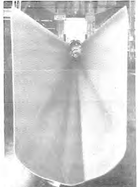
In one of the first stages in pipe making, this "U" shaped steel plate is squeezed in a matter of seconds into an "O" length of pipe.
