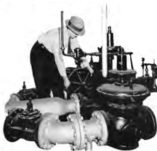
These enormous pressure regulators control the natural gas entering Shell Chemical's Gas Reform Plant.
