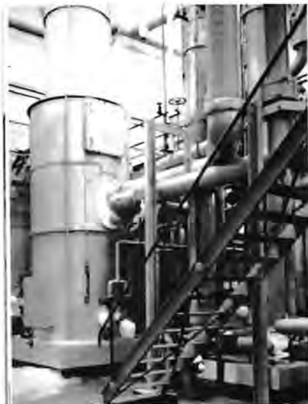
Nitrogen exists in great quantities in the air, but it takes this Linde apparatus, operating at 380° below Zero, to get it out.
